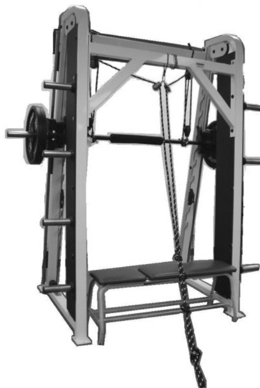
Figure 1. Modified Smith rack. A traditional Smith rack was modified with pulleys in order to isolate the eccentric and concentric muscle actions during the parallel knee squat exercise.
