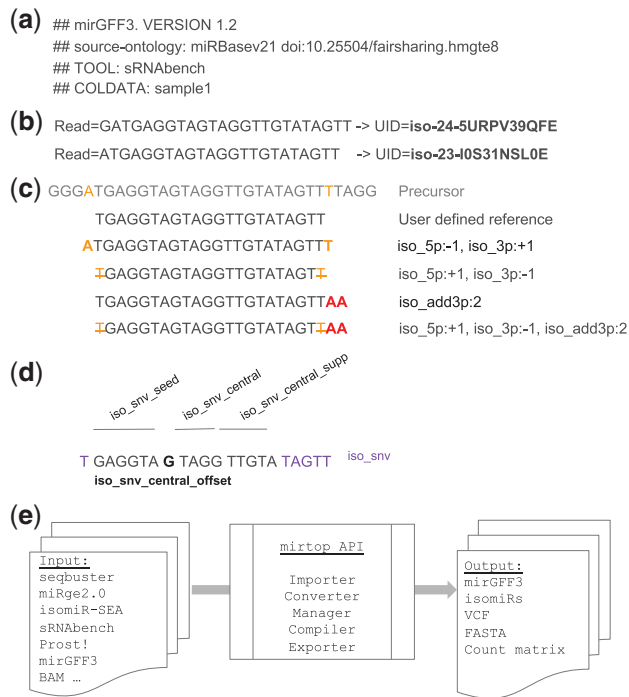
Fig. 1. The mirGFF3 file format and the mirtop API. (a) Example of input file header and the required lines: file format version, database used and samples included. (b) Examples of sequence compression to uniquely identify each sequence. (c) Examples of isomiRs with changes at the 5'- and 3'-ends and their respective variant attributes. The first sequence represents a portion of the miRNA precursor (i.e. pre-miRNA) and the second sequence is the reference isomiR defined by the user or the database used. Bold orange letters indicate templated additions. Bold red letters indicate non-templated additions at the 3'-end of the isomiR. Orange strikethrough letters indicate non-templated nucleotide additions at the 3'-end of the isomiR. (d) Example of nucleotide changes at different positions/regions of the isomiR and their respective naming. (e) The mirtop API workflow shows the main formats accepted as input files, the functions the Python API have implemented and the output file formats
