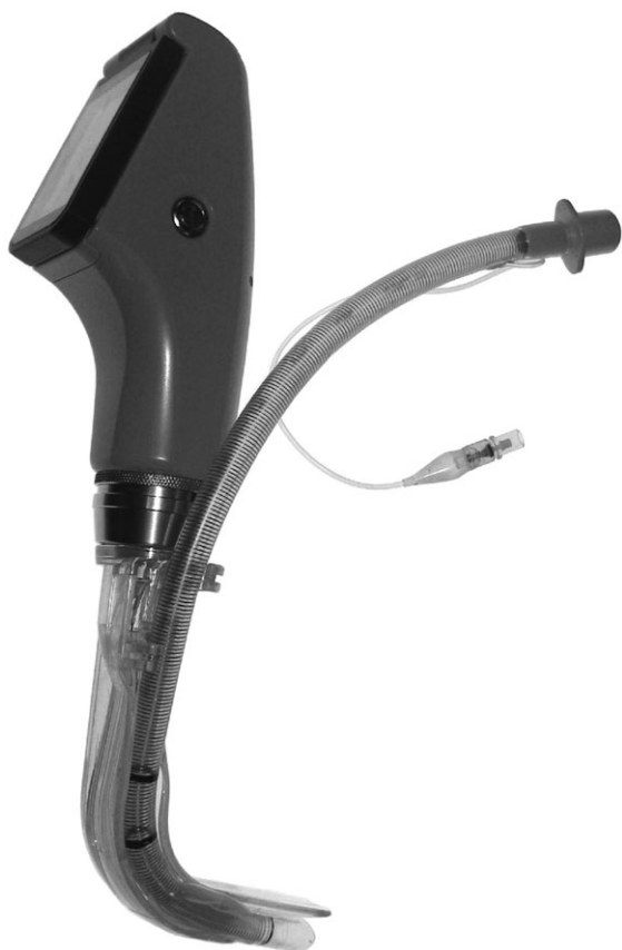
Fig 1 The Pentax-AWS (Tokyo, Japan). It consists of a disposable transparent blade (PBLADE®), a 12 cm cable with a CCD camera, and a 2.4-in. full-colour LCD monitor display.
