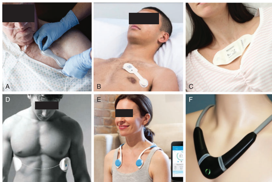
Fig 4 Examples of wearable and wireless sensors. Medical grade adhesive patches (A from VitalConnect, San Jose, CA, USA, B from Isansys, Abingdon, UK, C from Sensium, Abingdon, UK and D from Intelesens, Belfast, Northern Ireland) and necklaces (E from CloudDX, Kitchener, Canada and F from toSense, San Diego, CA, USA) designed to monitor heart rate, respiratory rate, thoracic fluid content, temperature and/or activity in ambulatory patients.
