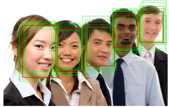
FIGURE 1. Visualization of the NMS process for a CNN-based face classifier (pre-NMS, light boxes; post-NMS, bold box).
