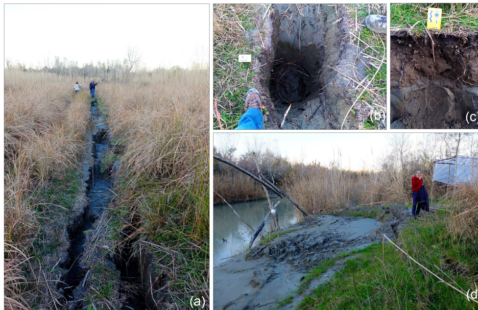
Figure 12. Site 10 of Fig. 8. Dozens of metres long fractures, opened up to 50 cm and associated with liquefaction, follow the left river bank of the Erzen River, affected by liquefaction and lateral spreading phenomena. (a) Panoramic view of one strand of these fractures. (b) Detail of a liquefaction conduct inside the fracture. (c) Side of a fracture showing the stratigraphy, with the soil above the clayey silts. (d) Lateral spreading of the Erzen River bank collapsed by liquefaction.
