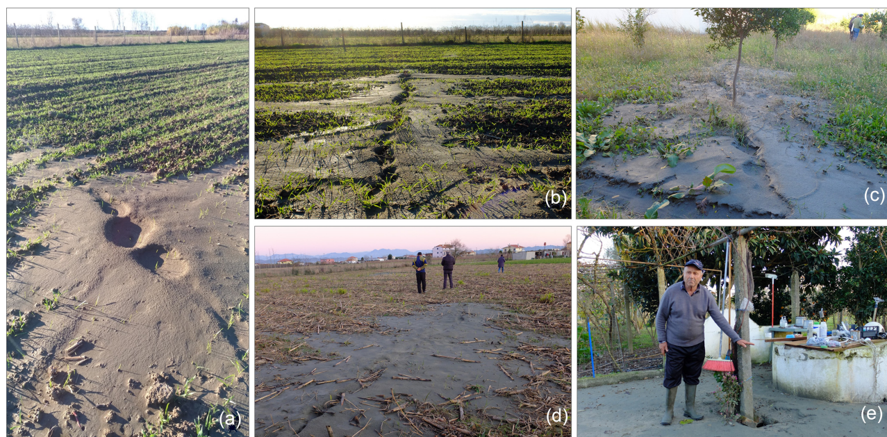
Figure 13. Liquefaction effects in the surroundings of Juba village. (a) Coalescent sand volcanoes; (b), (c) and (d) fractures with mounds of grey sandy silts on both rims. (e) Water and sand erupted up to a height of 1 m from a hole in the ground close to a water well. Site 11 of Fig. 8.
