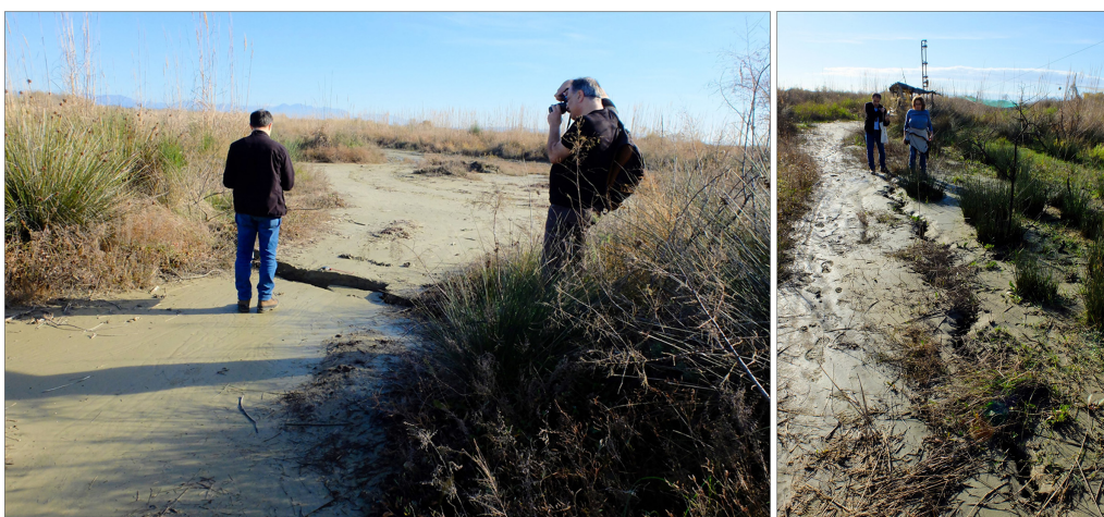
Figure 11. Site 9 of Fig. 8: Ground fracture (left-hand panel) induced by the Erzen river bank failure, with a 10–15 cm vertical throw lowering the side towards the river, and (right-hand panel) crack with ejected liquefied sandy silt. Cracks were up to tens of metres long.
