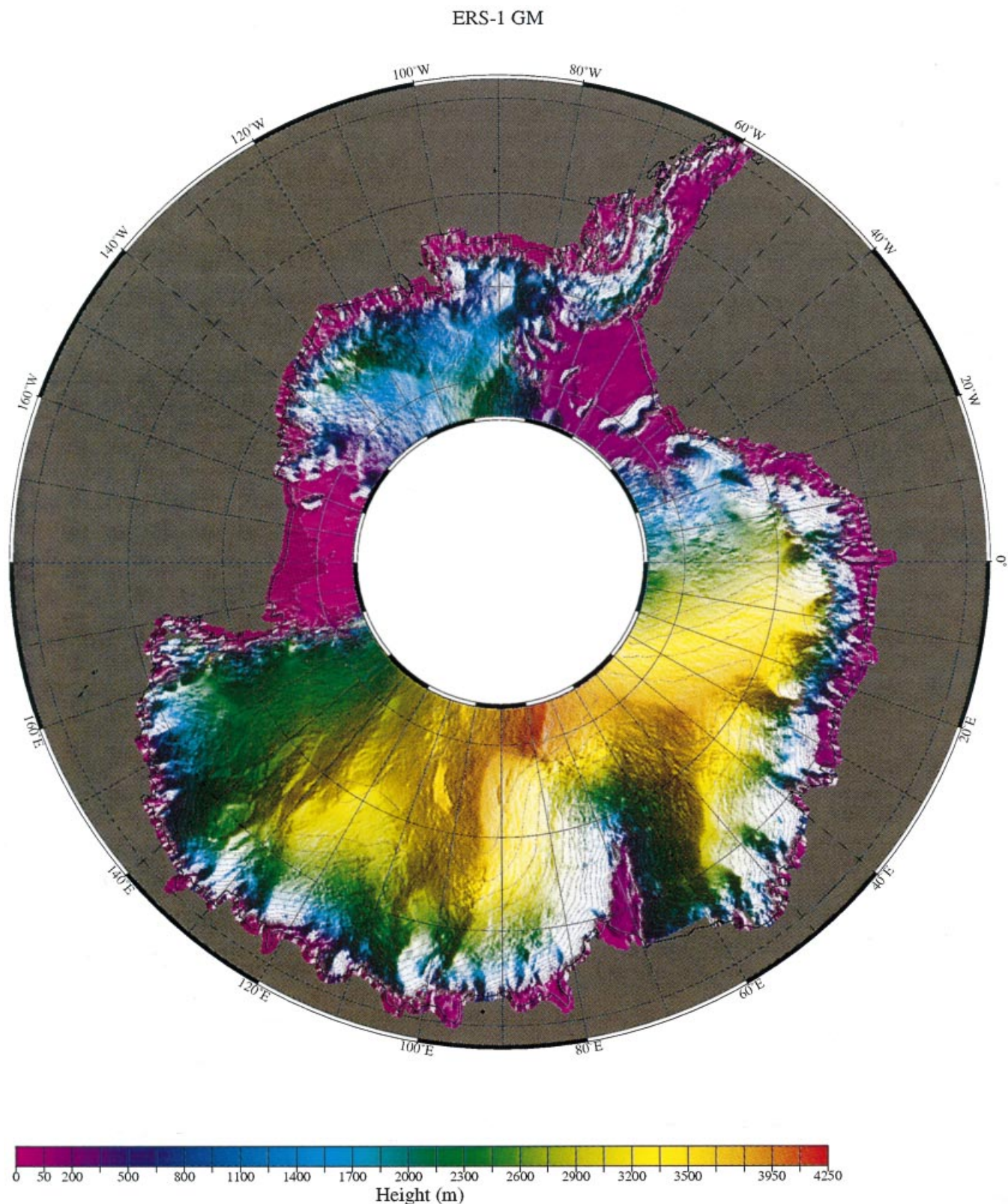
Figure 1. High-resolution map of Antarctic Ice Sheet topography from the ERS1 geodetic mission. The grid size is 1/30^\circ .
