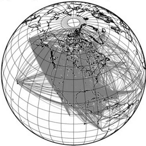
Figure 11. Path coverage for (a) the fundamental-mode Rayleigh wave at 76.9 s and (b) the second higher mode Love wave at 100 s.
