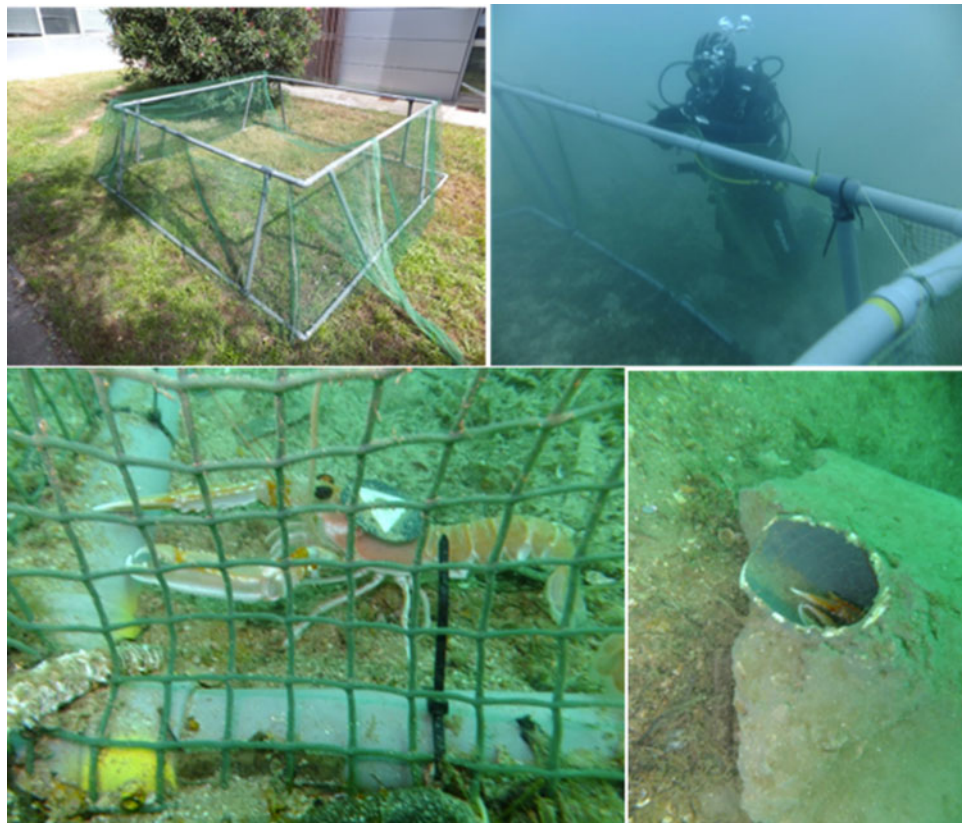
Figure 4. The OBSEA trials (Vilanova i la Geltrú, Spain) for the video monitoring of Norway lobster ( Nephrops norvegicus ) behaviour. Top left: cage to prevent animals escaping from the camera field of view. Top right: deployment and installation of the cage in front of the video camera. Bottom right: animal inside the cage with a plastic tag used for its identification. Bottom left: animal inside the artificial (PVC plus concrete) burrow.
