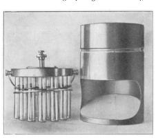
bands. The plate consists of two parts which can be moved by turning the head of the stem which comes up through the lid. If the head is slightly pressed down at the same time, only the inner portion, carrying the standards moves, if it is slightly raised, both parts will move.
