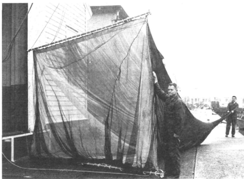
Figure 1. Beam trawl for zooplankton ( Calanus finmarchicus ), opening 4 \times 3 m, with protecting net.
