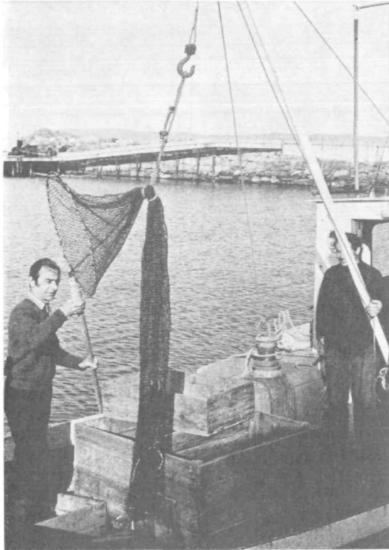
Figure 6. Lift net to heave the cod end of Calanus traps in case of large catches.
