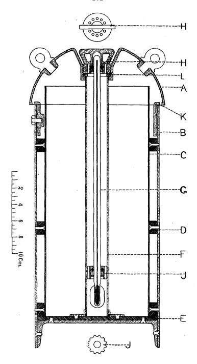
The water flows round the bulb of the thermometer and passes through ports in the tube (F) and so into the cavity of the body. When this is filled, the water leaves the apparatus through a series of ports (K) on the under-side of the head.
