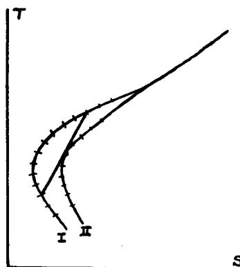
by drawing a tangent to the inner curve at the point of greatest curvature, thus cutting off an arc from the outer curve. The depth difference represented by this arc gives the value  $s$  in the formula:—
