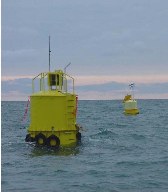
Figure 3. University of New Hampshire feed buoys for cod (left) and haddock (right).
