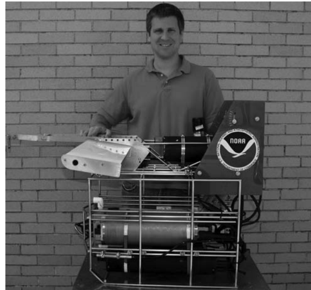
Figure 4. The Mariner Shuttle Mk II (MS Mk II) is based on the versatile Sea Sciences Acrobat towed body. Operation and on-board instrumentation is described in text.
