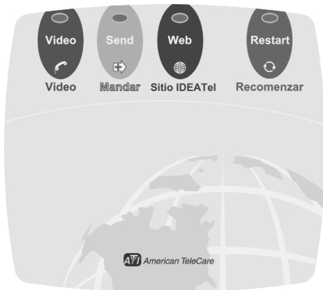
Figure 3 Patient launch pad. To simplify operation of the home telemedicine unit (HTU), a customized mouse pad was developed. The buttons are programmable function keys that allow patients to answer video calls or electronically transmit glucose and blood pressure readings with a single push of a button. Pressing the “Web” button will dial the Internet service provider and connect to the project Web site. The patient can then enter a password to view results. The “Restart” button allows the user to either reboot or shut down the system entirely.
