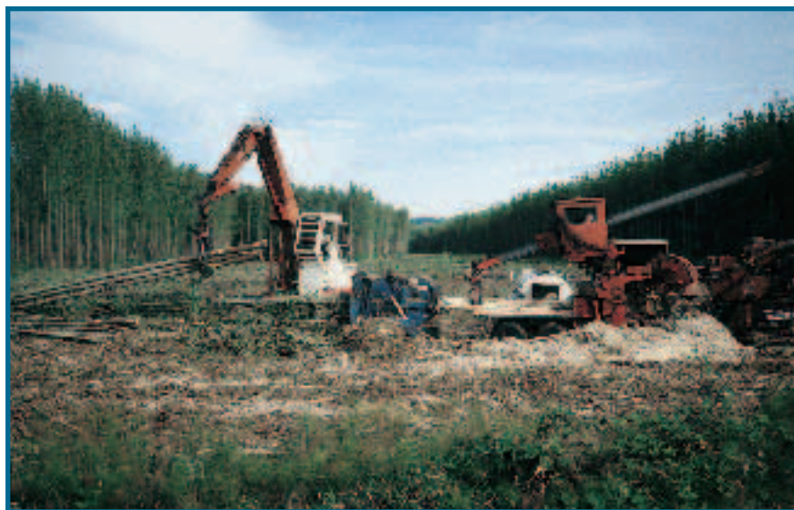
In-field delimiting, debarking, and chipping of trees from an eight-year-old hybrid poplar stand along the lower Columbia River floodplain. The yield of clean wood chips is 40 bone-dry tons per acre.
