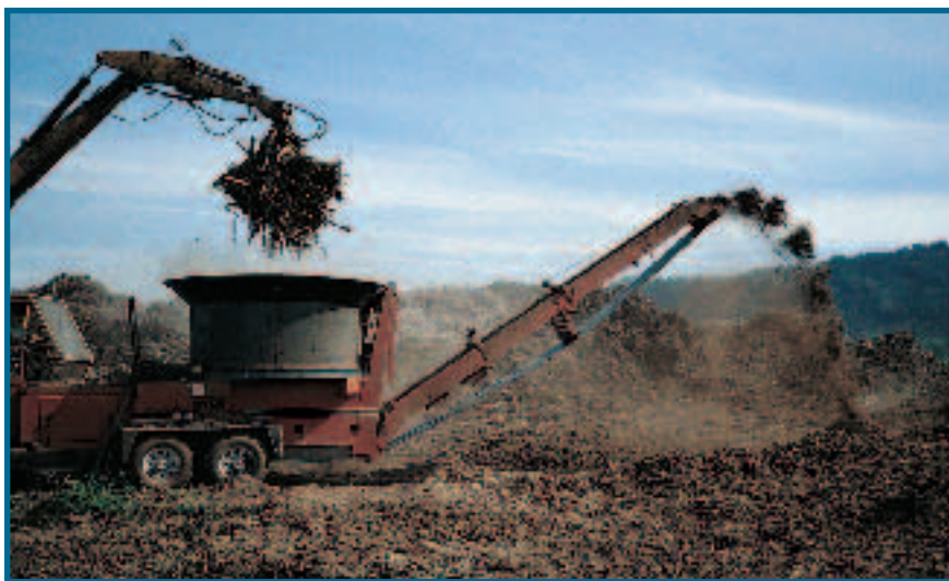
Hog fuel is ground for use in cogeneration boilers. Multiple markets, including energy feedstock, are important to the future profitability of hybrid poplar plantations.
