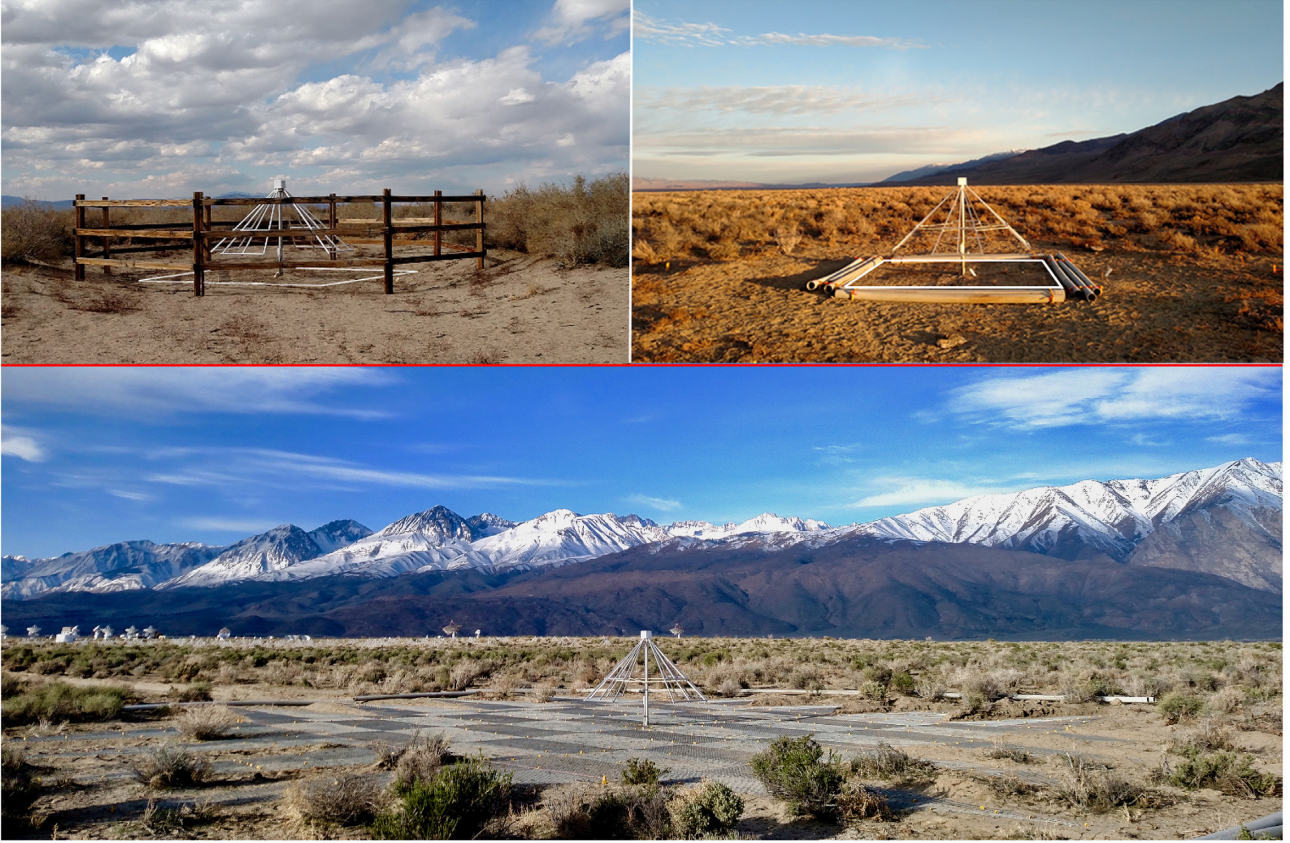
Figure 2. LEDA antenna 254, which sits in a slight depression surrounded by \sim 1 m-high woody vegetation (top left-hand panel), 252 prior to January 2019 (top right-hand panel), and 252 after (bottom) completion of the serrated ground screen in early 2019 April. Serrations that most strongly affect data were completed in February. The smaller ground screen (top figures) is 3 \times 3 m 2 (white boundary lines are intended to guide the eye) and flat to 10 cm peak to peak. The larger ground plane (bottom) is 20 \times 20 m 2 tip to tip and flat to 3 cm peak to peak. The antenna structure is aligned to within 1^\circ of true north and the antenna mast stands within 1^\circ of vertical. At antenna 252 (top right-hand panel), PVC pipes were used as a cattle guard in place of wood fencing because water absorbed from rainfall by the wood has the potential to affect the antenna gain response.
