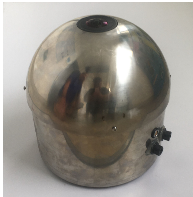
Figure 1. A photo of KLCAM. On the top is the camera lens. The sockets on the side of the metal shell are for the network connection and power supply.
