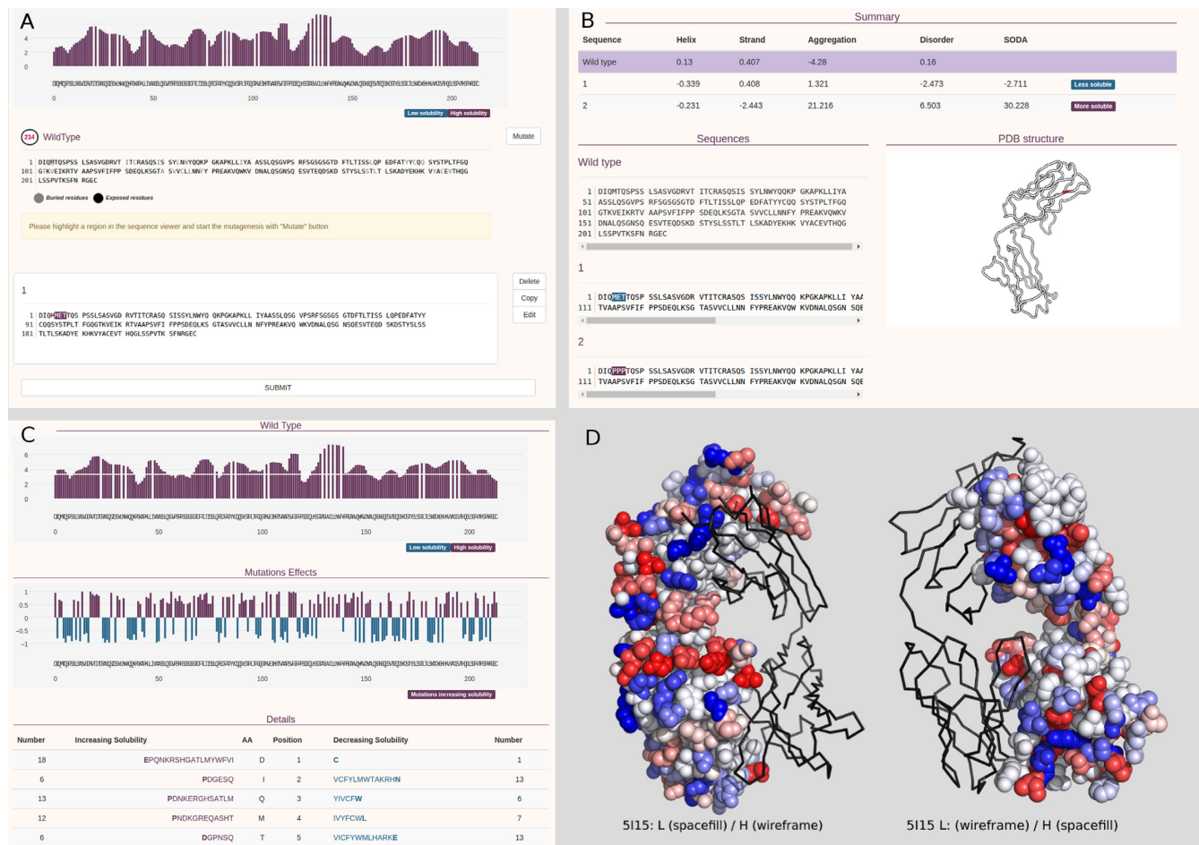
Figure 1. Sample SODA mutation and result pages. (A) The mutation input page is returned when the user chooses ‘mutation mode’. It allows to create multiple instances of mutations/deletions/insertions. (B) The ‘mutation mode’ result reports changes of the protein solubility upon mutation. When a PDB is provided as input the mutated region is highlighted in the structure. (C) The ‘full protein mode’ provides the solubility profile (first plot) and the propensity of increasing or decreasing solubility for all sequence positions (second plot and table). (D) The human germline antibody IGHV1-69/IGKV1-39 (PDB code 5i15) is shown alternatively as wireframe and space fill between light (L) and heavy (H) chain. For each position, the probability of increasing (red) or decreasing (blue) solubility upon mutation is mapped on the structure. On the left, the light (L) and heavy (H) chains are shown as wireframe and space fill respectively, on the right the same protein with opposite chain visualization mode is provided.
