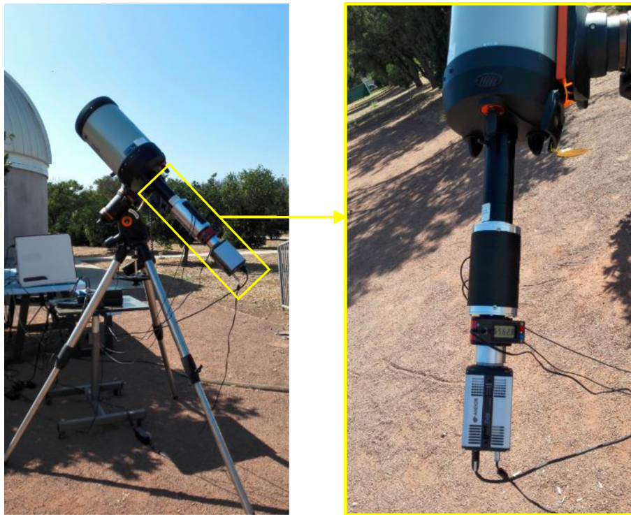
Fig. 8. HIPO system mounted to a 200-mm H\alpha solar telescope for polarimetry observation. (Color online)
