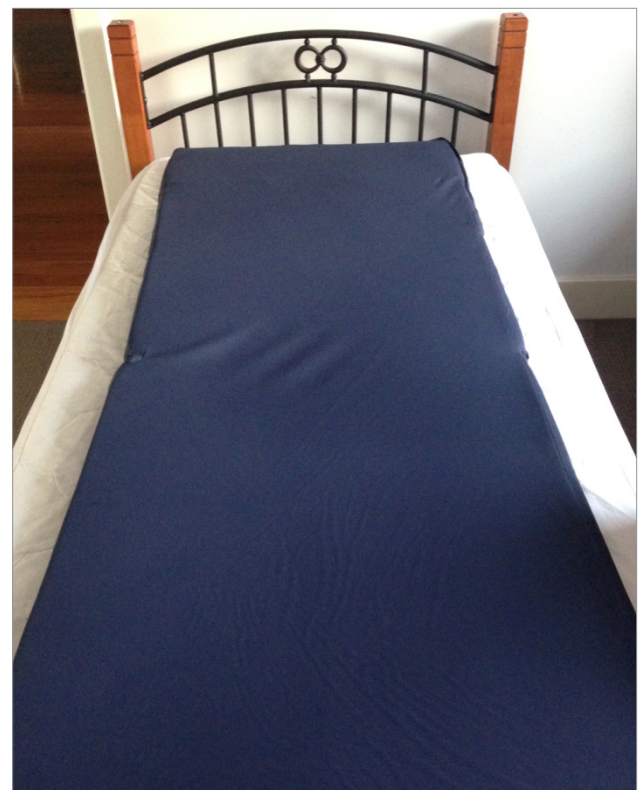
Figure 2 —Photograph of the Sonomat positioned on a bed. During the night, a bedsheet completely covers the Sonomat, and this sheet is tucked under the existing mattress with all other bedclothes arranged as normal.
