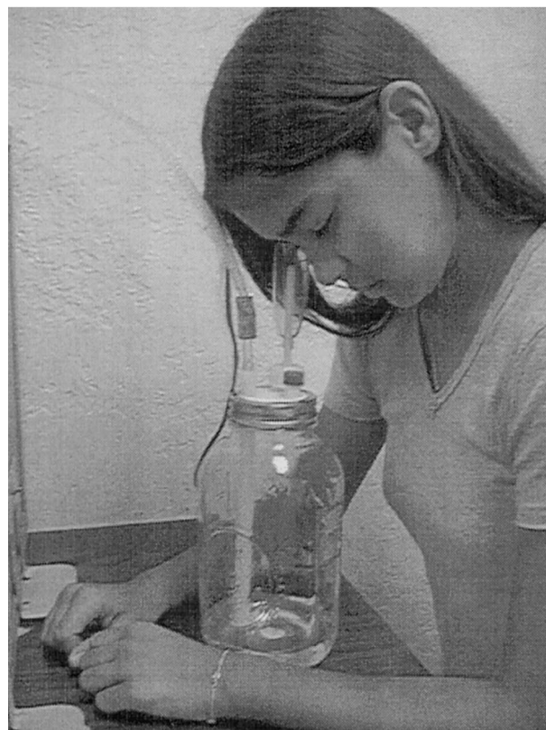
FIG. 1. (Top panel) Picture of the glass vessels with the eyepiece adapted. (Bottom panel) Picture of a subject being tested for eye irritation with the glass vessels.
