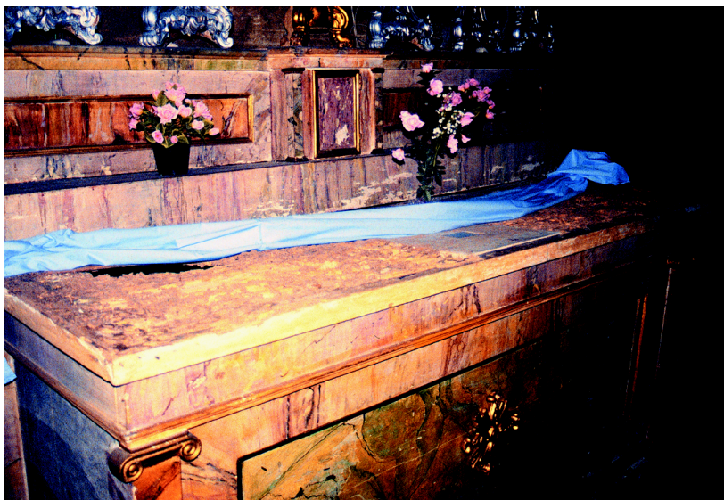
Fig. 8. Altar table of a historic church in northern Italy that had been severely damaged by termites. The church was treated with liquid insecticides for years, but the infestation continued.
