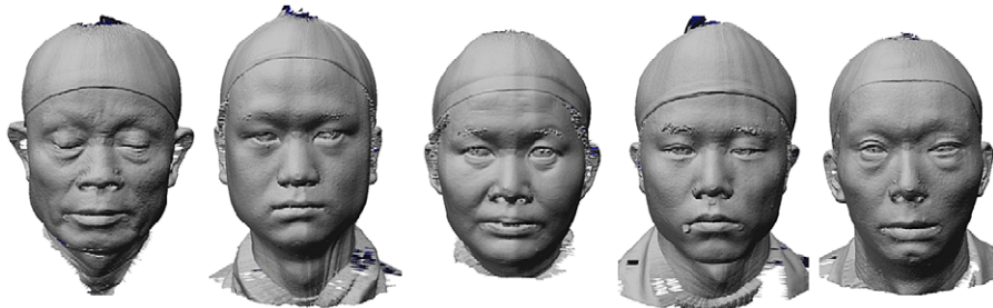
Fig. 5. Images of the scans for subjects chosen to construct the medium headform.
