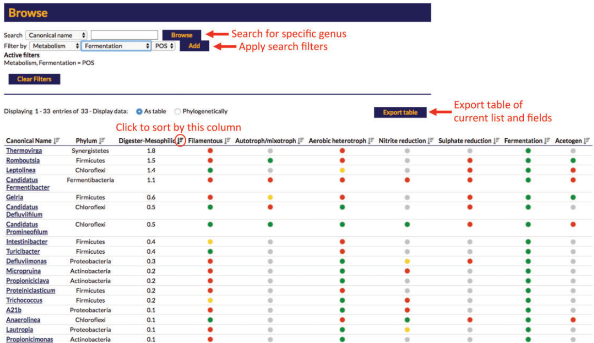
Figure 6. Screenshot of the result displayed from a search of the online MiDAS database. The displayed example is applying a search filter for fermentative organisms sorted by median read % abundance in mesophilic anaerobic digesters. Select features are highlighted in red.
