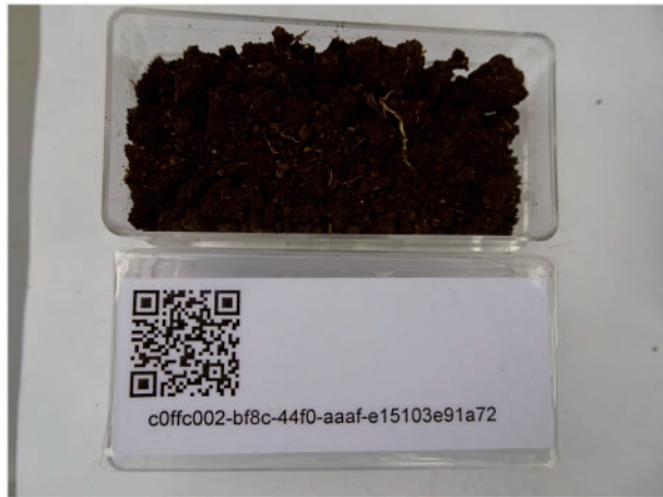
Figure 2. UUID-QR labelled box with soil sample being imaged at the sampling site Ruma (Kenya) with a digital camera with GNSS resp. GPS functionality.
