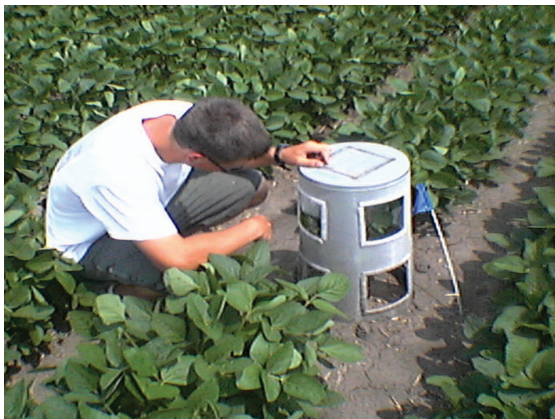
Fig. 1. Cage with open windows to permit ingress and egress of arthropod natural enemies.
