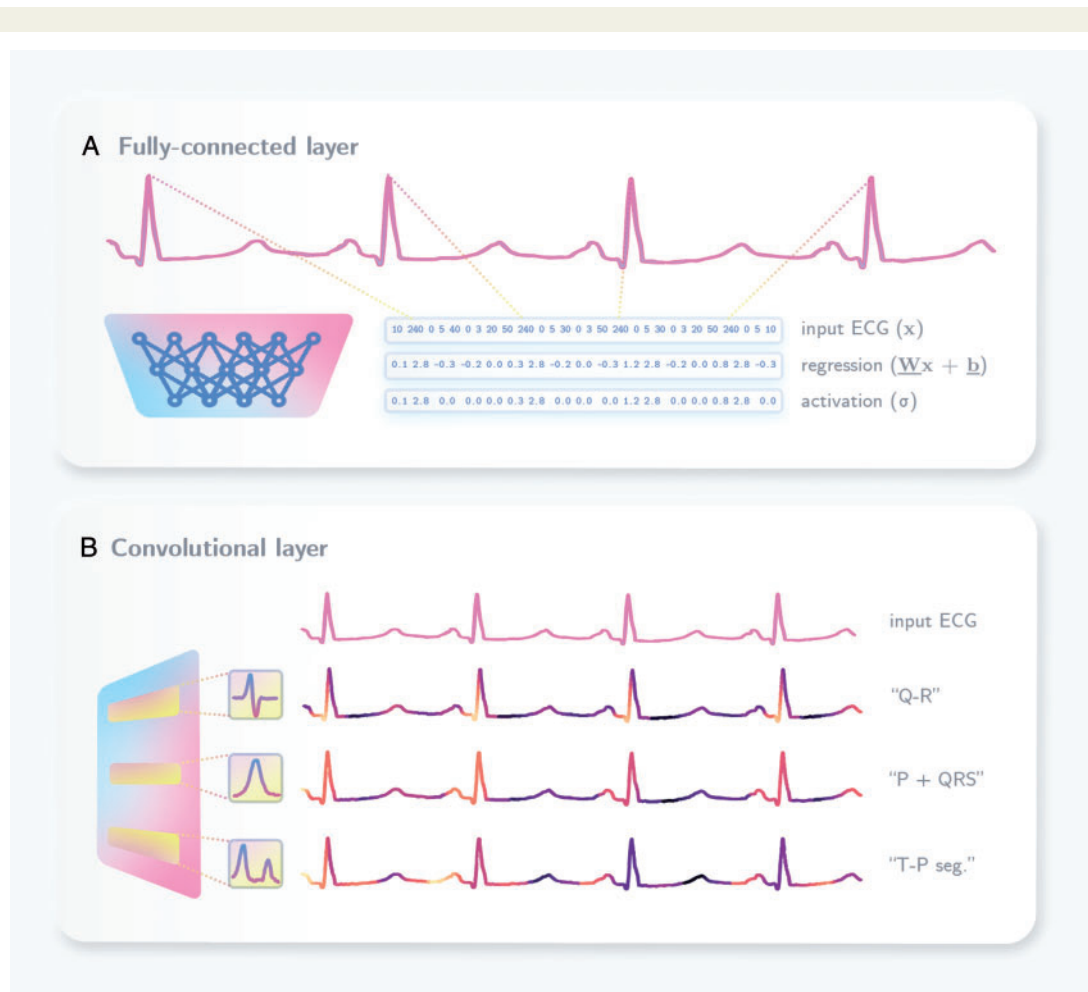
Figure 1 Understanding important layer types. Two common layer types used in deep learning pipelines for image processing are fully connected layers (top), which function simply as many linear regression models with a non-linear activation function that increases the informational capacity of the model. Convolutional layers (bottom) are composed of many ‘kernels’ that learn particular patterns to pick up (small gradient boxes) and scan across an input signal where that pattern may be present. In this example, the kernels from the top to below represent the shape of a R-S wave, a P-wave, and T-P wave segment, and their relative strengths of detection (high: yellow, low: blue) are shown for the input ECG signal (magenta). The resulting signals demonstrate localization of these key kernel patterns that helps the deep learning model learn both the presence and relationship of such features in the input signal. ECGs, electrocardiograms.
