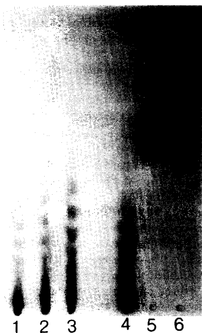
Fig. 3. Thin-layer chromatography of the products of xylan hydrolysis by purified xylanase. Lanes 1, 2, 3 and 4 are from 10-, 30-, 60- and 1440-min samples, respectively. Lanes 5 and 6 represent xylobiose and xylan standards, respectively.
