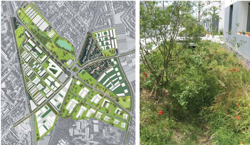
Figure 3. Project map of the urban planning of ecoquartier Bottiere-Chenaie in Nantes (left); vegetated ditch receiving runoff rainwater coming from streets and houses (right).
