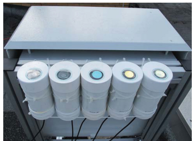
Figure 2. Prototype detector set-up. Five SQMs are securely fixed to a weatherproof box, which contains the acquisition computer. Each of the SQMs views the sky through a different filter: from left to right the standard SQM filter, a luminous filter, and red, green and blue filters. (The red filter appears blue in the photo because the red light has been transmitted and absorbed at the detector.) After this photo was taken, an IYA lightmeter was attached to the top left side of the weatherproof box.
