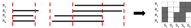
Figure 4. The segmentation is projected on the reads. Each read is represented as a binary vector of size equal to the number of canonical segments. A segment has a value of 1 (filled grey) if a read has at least 90% coverage over the segment, and 0 otherwise.
