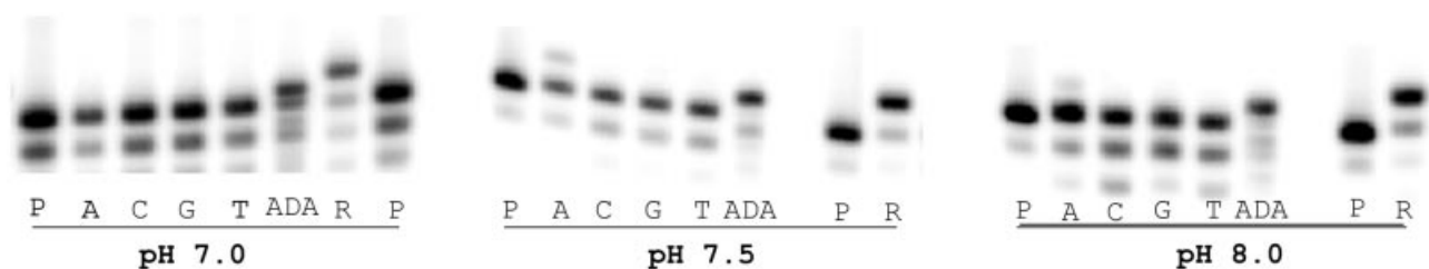
Figure 4. Single nucleotide primer extension experiments as a function of pH with Y188L. Variant Y188L was incubated for 30 min at the pH indicated, with template T2-pyDAD, radiolabeled primer P2-SS and one of the four standard deoxynucleoside triphosphates or d(puADA)TP. Lane P, primer alone; lane A, with dATP; lane C, with dCTP; lane G, with dGTP; lane T, with TTP; lane ADA, with d(puADA)TP; lane R, positive control with substitution of T2 for T2-pyDAD, thus having dA instead of the non-standard nucleotide. Noticeable in all experiments is the primer band (labeled P) and a degradation band (below the primer band); the degradation of the primer was due to a DNase activity of the RT itself, an activity that was removed by the mutation E478Q (see text). Little incorporation was observed at pH <6.5; the optimal pH was 7.0–7.5. It should be noted that oligonucleotides containing a puADA residue migrate slightly faster due to the negative charge on the heterocycle.
