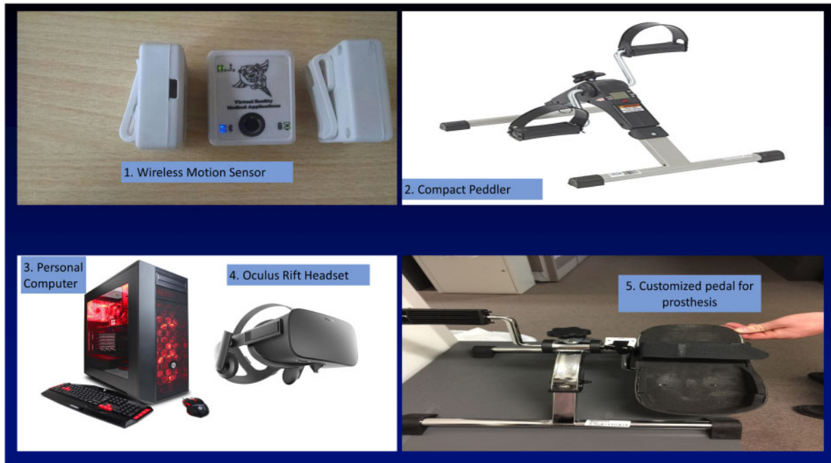
Figure 1. Illustration of the virtual reality treatment hardware, consisting of a motion sensor, bicycle pedaler, computer, Oculus headset, and prosthetic pedal.
