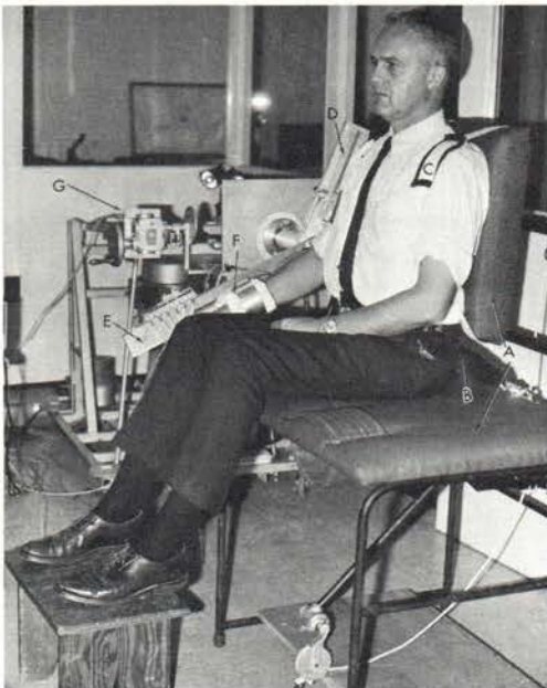
Fig. 1. Normal subject positioned for measurement. A. Adjustable positioning bench. B. Seat belt. C. Shoulder harness. D. Stabilizing arm. E. Rotating arm. F. Multicompartment inflatable wrist cuff. G. Adjustable base.
