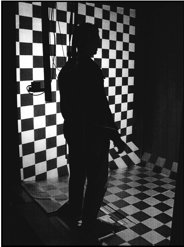
Figure 3. Silhouette view of a person demonstrating the use of the Balance Near Automatic Virtual Reality Environment (BNAVE) laboratory with the checkered optic flow stimulus. The patient is standing on a movable force platform, and an electromagnetic motion transmitter is behind the patient.
